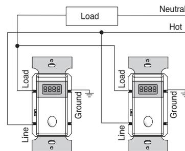
When using a three-way application, lights may be turned on from either switch, but can only be turned off at the switch that turned them on.
