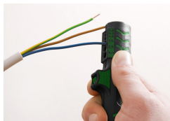
Stripping a wire insulation.
