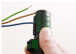
Stripping a wire insulation.
