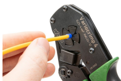
Squeeze handles until ratchet mechanism is released.
