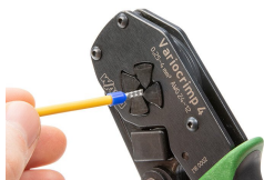
Insert the ferruled conductor into the crimping station.
