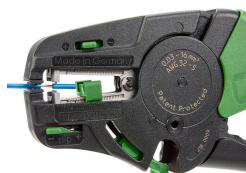
Partially stripping a conductor.
