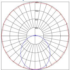
Maximum Candela = 1870.9 Located At Horizontal Angle = 22.5, Vertical Angle = 1 # 1 - Vertical Plane Through Horizontal Angles (22.5 - 202.5) (Through Max. Cd.) # 2 - Horizontal Cone Through Vertical Angle (1) (Through Max. Cd.)
