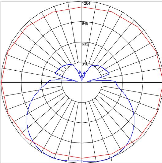
Maximum Candela = 1264.2 Located At Horizontal Angle = 0, Vertical Angle = 16.5
