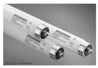
OCTRON 8-ft FO96/800/XP/ECO lamps can be used to replace FO96/700 or FO96/800 lamps to increase initial and maintained light levels and provide 20% longer lamp life. The CRI of 85 means excellent color rendition. Three different color options are available: 830 with a color temperature of 3000K, 835 with a color temperature of 3500K, and 841 with a color temperature of 4100K.
