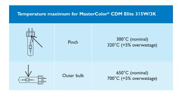
Temperatures are measured on burning lamps. Exceeding the maximum temperature will not guarantee optimal performance (lifetime, lumen maintenance).
