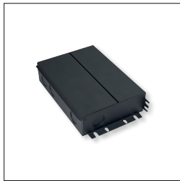
Class II Universal Dimming Driver NPSU-60W/24 60W NPSU-96W/24 96W NPSU-3X96W/24 3x 96W Input Voltage: 110-277V Dimming: Triac, ELV, MLV, 0-10V, PWM Note: Power Line Connector(s) not included
