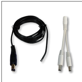
Power Line Connector NALT-10 10' Power Line NALT-30 30' Power Line For use with Class II drivers. Carries output from driver, requires power line interconnectors. NATL-302W 5" Splitter Splits power line connector into two separate leads, requires power line cable.
