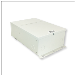
Class II Hardwire LED Driver with Breakers, MLV Dimming NMT-303/24C2D1 120V input NMT-303/24C2D2 277V input Input Voltage: 120V or 277V Dimming: Magnetic Low Voltage Breakers: (3) 100W Note: Power Line Connector(s) not included
