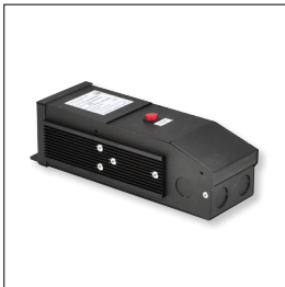
Class II Hardwire LED Driver with Regulator, MLV Dimming NMTD-60/24D 24V 60W NMTD-96/24D 24V 96W Input Voltage: 120-277V Dimming: Magnetic Low Voltage Regulator: Integral regulator for constant current and voltage Includes: 10' Power Line Connector
