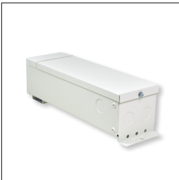
Class II Hardwire LED Driver MLV Dimming NMT-48/24C2D1 48W Input Voltage: 120V Dimming: Magnetic Low Voltage Includes: 10' Power Line Connector
