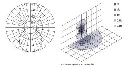
Fixture tested per LM-79-08. Photometric data is of the performance of a representative fixture. Results may vary in the field.
