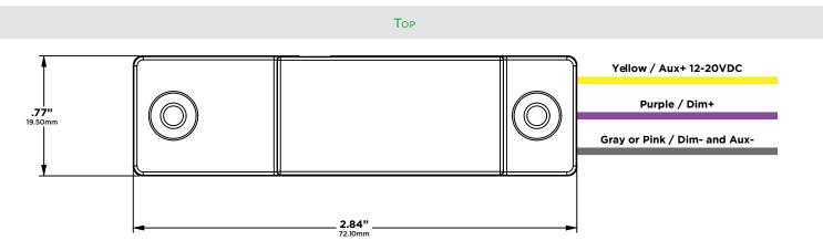
Connect the Gray/Pink wire to DIM- and AUX- together if a separate AUX- is present in the LED driver.
