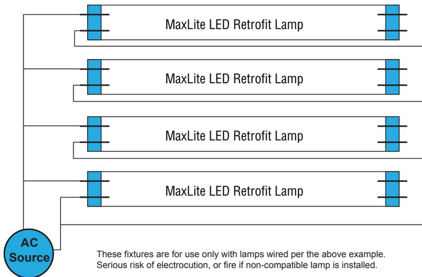
These fixtures are for use only with lamps wired per the above example. Serious risk of electrocution, or fire if non-compatible lamp is installed.
