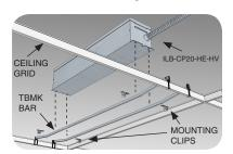
Use the TBMK mounting kit to remote mount flexed units within a grid ceiling. The ILB-CP is secured to the bars of the TBMK via mounting clips. The bars then mount to the T-bars of the ceiling grid. The flexible conduit of the ILB-CP connects to the fixture.
