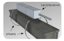
The strapping kit provides (2) straps that run through the mounting tabs of the ILB-CP for securing to a beam or column near the fixture. Overall strap length is 18".
