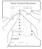
Note: If the Receiver has already been PC programmed it will return to normal operation after the LEDs flash rapidly for 10 seconds instead of entering APM.
