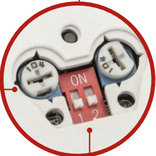
DIPSWITCH DIMMING ADJUSTMENT (50%, 25%, 10%, OFF)
