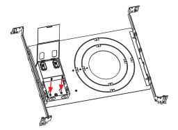
4. Place the plate between applicable joists where downlight will be installed; use a hammer to knock plate brackets into joists.
