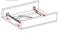
**5.** Once the plate is attached to joists, follow appropriate downlight installation instructions to complete the installation.
