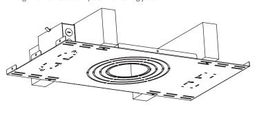
2. Secure plate to joists with appropriate screws (not included).
