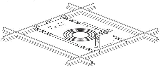
2. Secure plate to T-grid with appropriate screws (not included).
