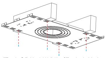
Note: Plate comes out of the box ready to be installed onto joists that have 12" or 16" spacing. To fit plate onto joists that have 24" spacing, simply bend down end tabs and screw to joists.
