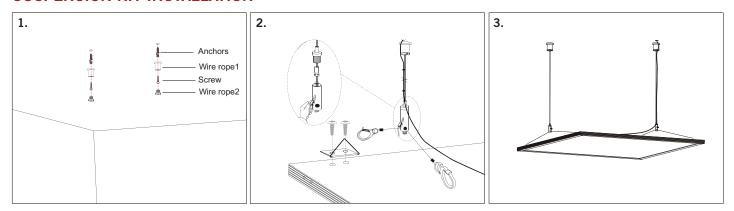
Note: Recommended 2 Cables for 2x2 and 1x4 Installations. 3 Cables for 2x4 Installations.
