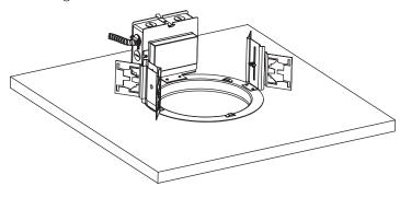
2. Attach one end of the KT-MC-NP-1-18/3 cable to the KO in the existing fixture J-box and connect the wires to the incoming power (L, N, G).
