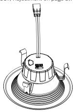
**4.** Plug E26 base cable connection into the recessed housing.
