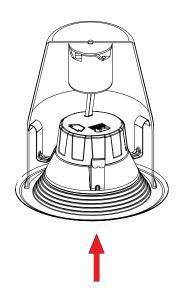
**6.** Push the LED trim into the housing until trim is flush with ceiling.
