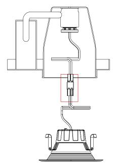
**5.** Carefully route wires into fixture, sliding the trim and friction clips into the housing.
