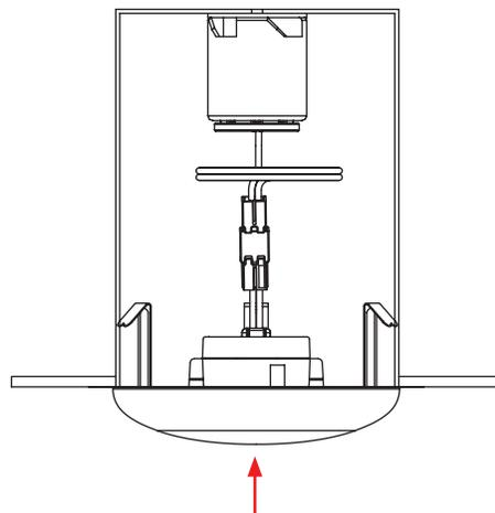
9. Push the disk light up until light is flush with ceiling.
