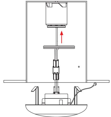
7. Secure fixture ground (green) wire to the recessed housing.
