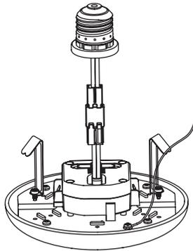
5. Select desired CCT using adjustment switch on disk base (see *Color Select (CCT) Adjustment* on page 3).
