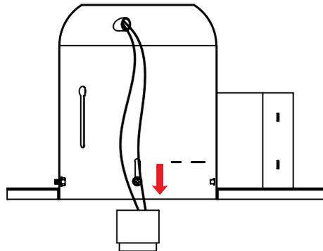
3. Remove existing socket mounting plate from the housing, then remove lamp socket from the plate.
