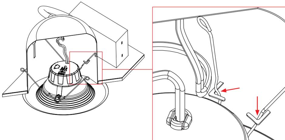
8. Carefully place wires into the fixture, then push the LED trim into the housing until trim is flush with ceiling.
