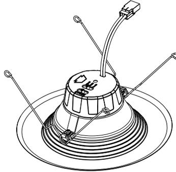
6. Plug E26 base cable connection into the recessed housing.
