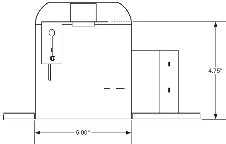
1. Shut off power at the source of the recessed housing into which you are installing fixture. Remove existing trim and CFL or incandescent bulb.
