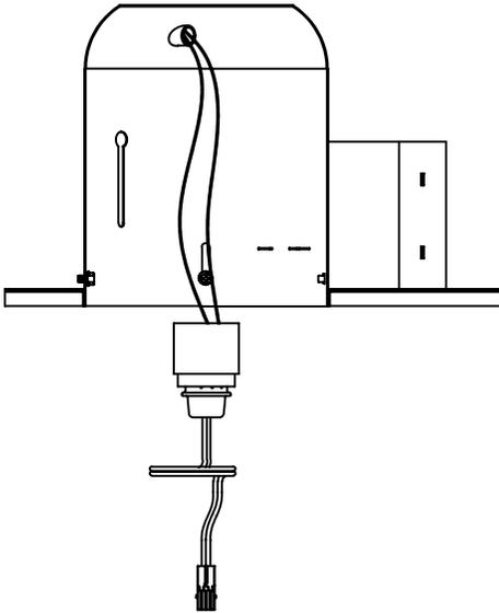
5. Select desired Wattage and CCT using adjustment switches on driver box (see *Power Select (Wattage) and Color Select (CCT) Adjustment* on page 3).
