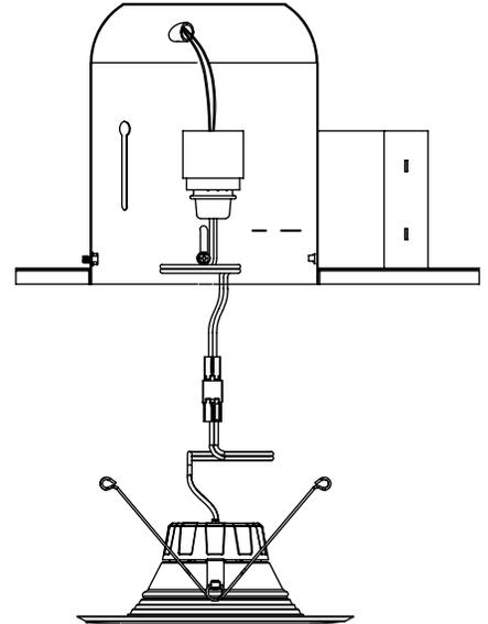
7. Squeeze torsion springs as shown and install into the metal brackets inside the recessed housing. For proper installation, the torsion springs should be seated within the brackets and on both sides of the housing.
