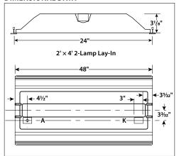
A: %" Diameter knockout K: 2" × 3" through hole for access plate.
