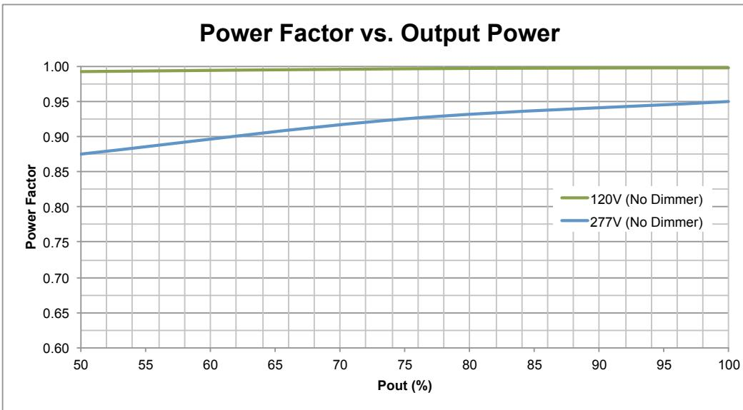
Efficiency and PF measured at 25°C.
