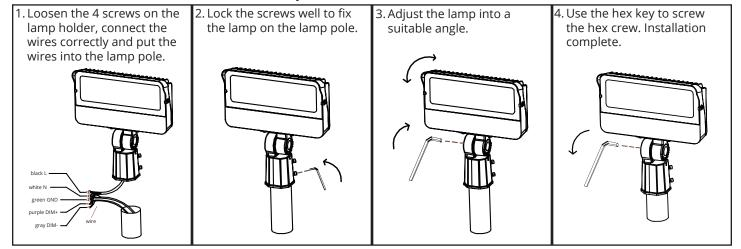
Notice: Locking bolt can be only compatible with a lamp pole that the outer diameter is Ø60, and lamp adjustable angle is 0-90°
