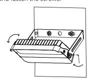
6. Fasten the screws to both sides with the allen wrench.
