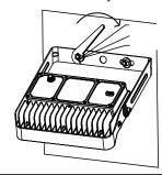
5. Rotate the light to the proper angle and fasten the screws.
