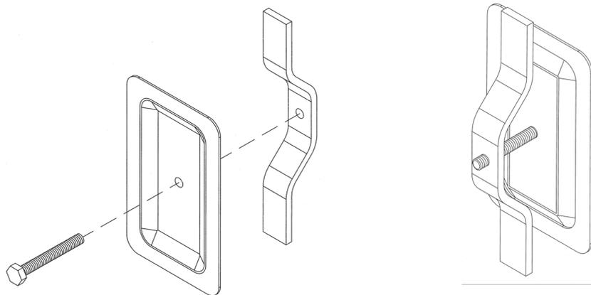
INSTALL MOUNTING BOLT (C) THROUGH THE COVER PLATE (A) AND THREAD INTO MOUNTING BRACKET (B) ALLOWING THE BOLT TO COME THROUGH ABOUT 1/4".
