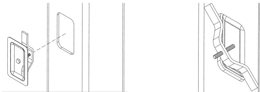
INSERT MOUNTING BRACKET INTO HAND HOLE. WHILE HOLDING COVER PLATE FIRMLY IN PLACE, TIGHTEN BOLT UNTIL COVER PLATE IS SECURE.
