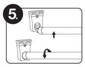
Install Bulbrite LED T5 DIRECT lamps.
