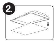
**Remove diffuser**In the case that diffuser is present.
