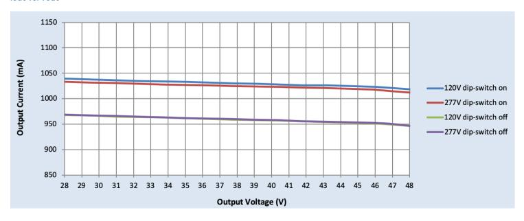
When designing LED board, please consider LED voltage increases due to cold temperature, forward voltage tolerance and aging to make sure LED voltage is always below 48V. Recommended typical LED voltage at room temperature 43V or below.
