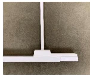
Install the Live End Connector and wire through the knockout then slide the cover (Part D) down to cover up the knockout. Then repeat instructions for the other end of the track.
