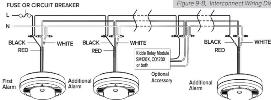
Figure 9-B, Interconnect Wiring Diagram
